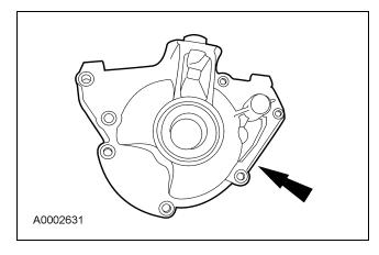
4. Inspect the case bearing for damage. If damage to the case bearing is indicated, install a new case.
